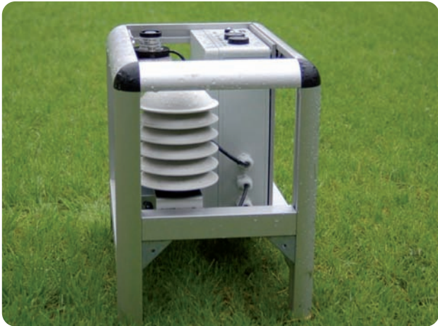
Grass Analyser portable stand.
